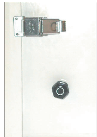
Above is a closeup of the SC-IRDA Interface mounted in an enclosure compression fitting. To communicate with the datalogger, point the PDA's IRDA sensor at the SC-IRDA sensor head exposed on the outside of the enclosure.
