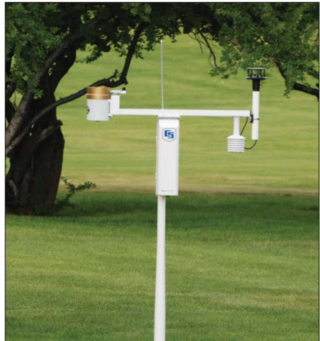
The ET107 provides real-time weather measurements and calculates ET o on an hourly and daily basis.
