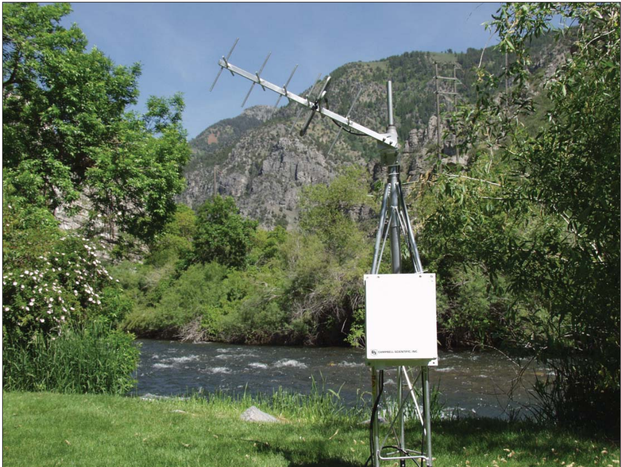
The DCP200 is intended for stream stage, water quality, and rainfall applications. The ENC16/18 environmental enclosure houses the DCP200's transmitter, datalogger and power supply.
