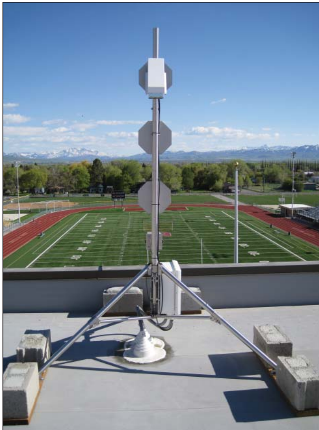
Logan High School in Logan Utah has installed a lightning warning system that includes the CS110. The CS110 is mounted to a CM110 10-ft stainless-steel tripod that sits on a roof next to the football field (left). Lights included in the system indicate the likelihood of lightning (right).
