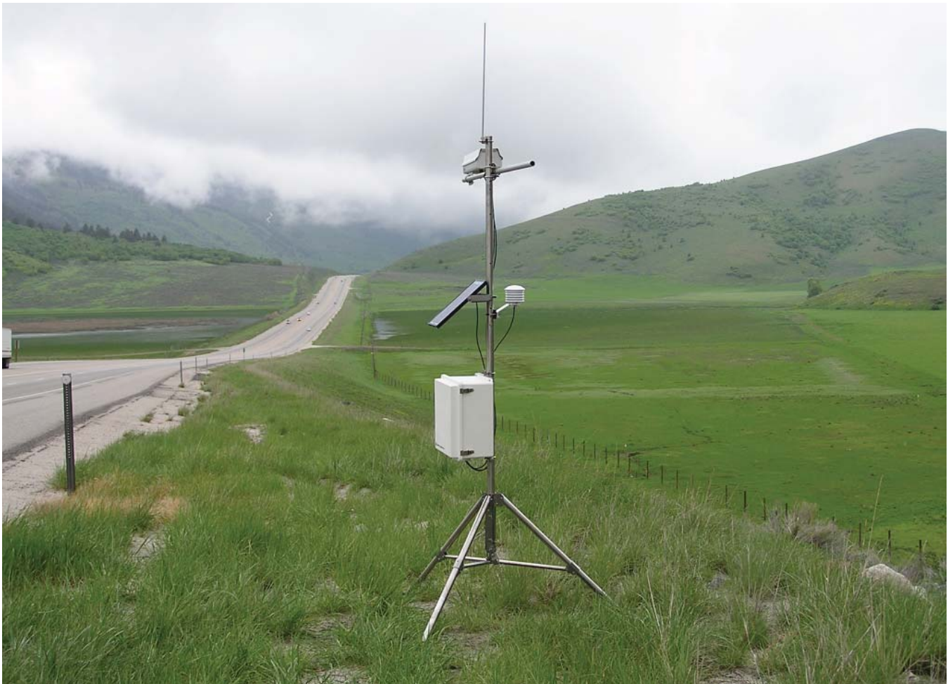
The CM110 10-foot tripod shown above is not guyed. An optional guy kit is offered for the CM110 if additional stability is required. A guy kit is shipped with the CM115 and CM120.
