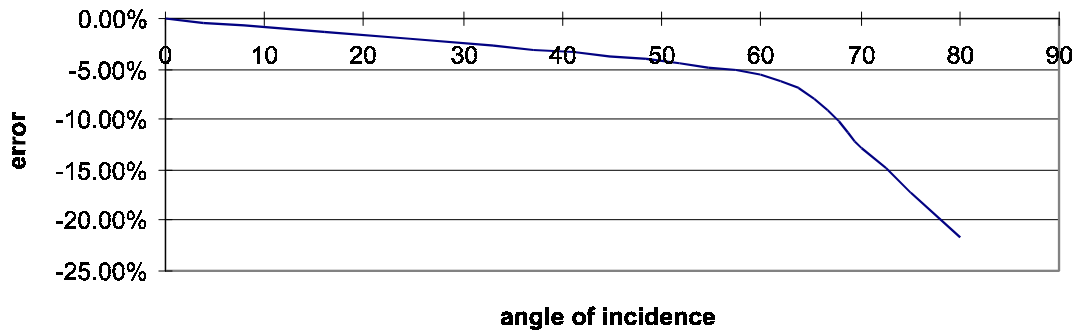
FIGURE 4. Cosine Response of a Typical Net Radiometer
